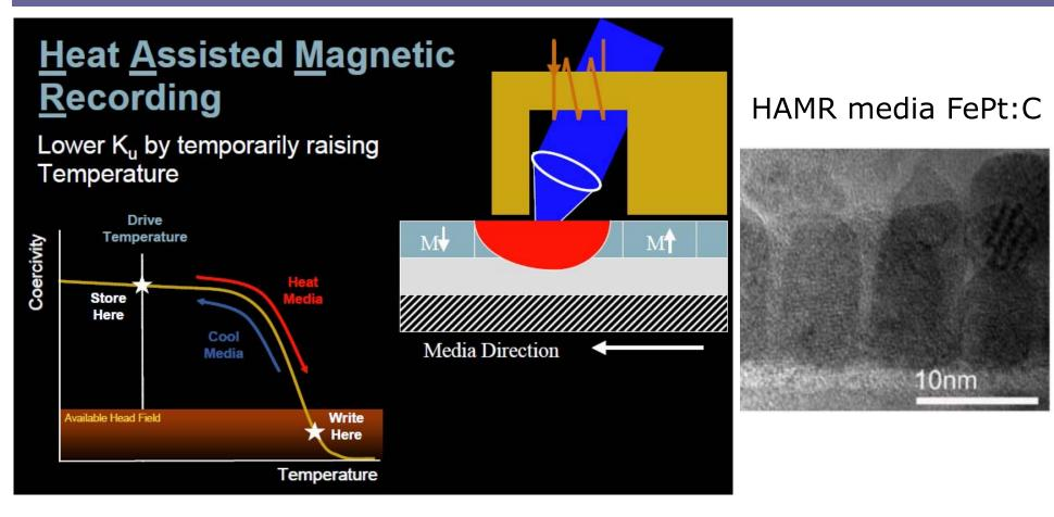
Velocity of media 10 m s<sup>-1</sup>. Size of bit 10 nm. Time-scale 1 ns.
