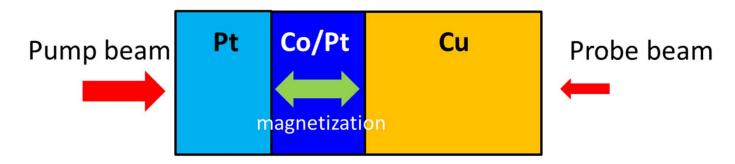
Sapphire/Pt(30)/[Co/Pt] $_{xn}$ (6)/Cu(10)/CoFeB(2)/MgO(10)/AlOx(5) (in nm)
